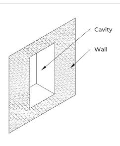
1. Make a cavity with an approximate size: 160 mm x 90 mm x 68-83 mm (length x width x depth)
